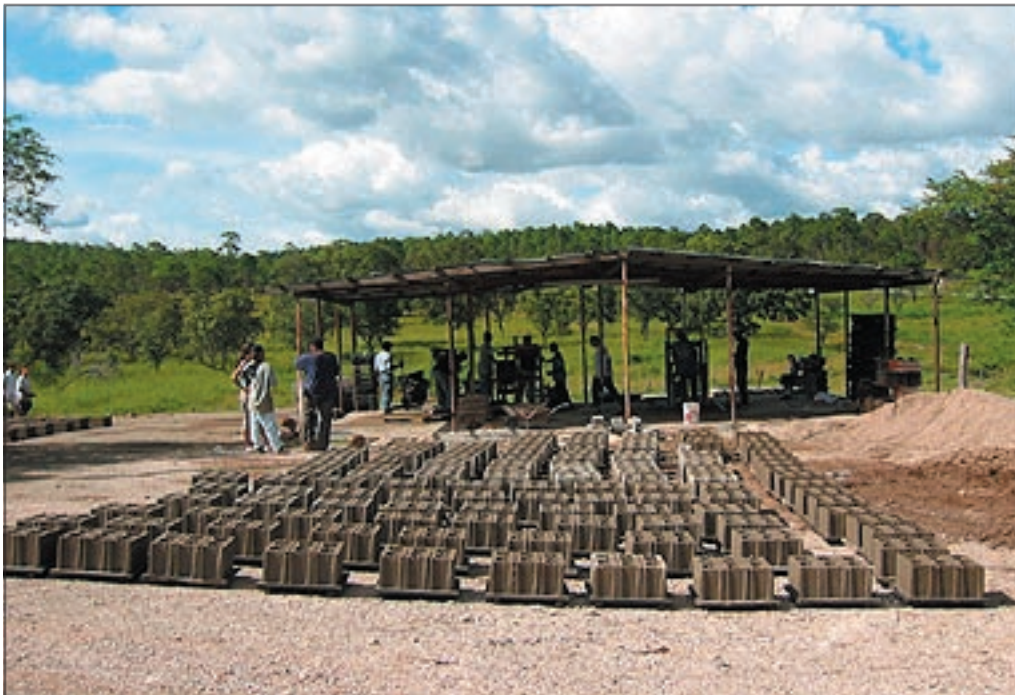
Our block factory. We produce about 400 blocks in five hours.
